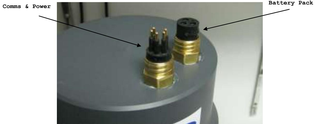
**Fig 5 - Electrical Connectors**
