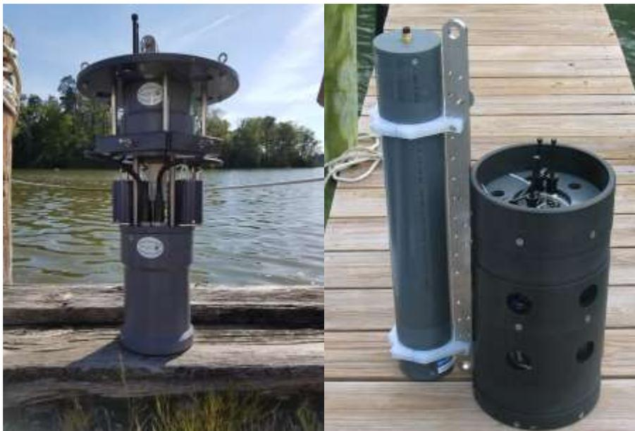
**Fig 3 - EcoLAB with reagent hanger and high sensitivity detectors (left) and EcoLAB mounted in reagent housing with battery pack, mooring tie bar and battery pack (right).**
