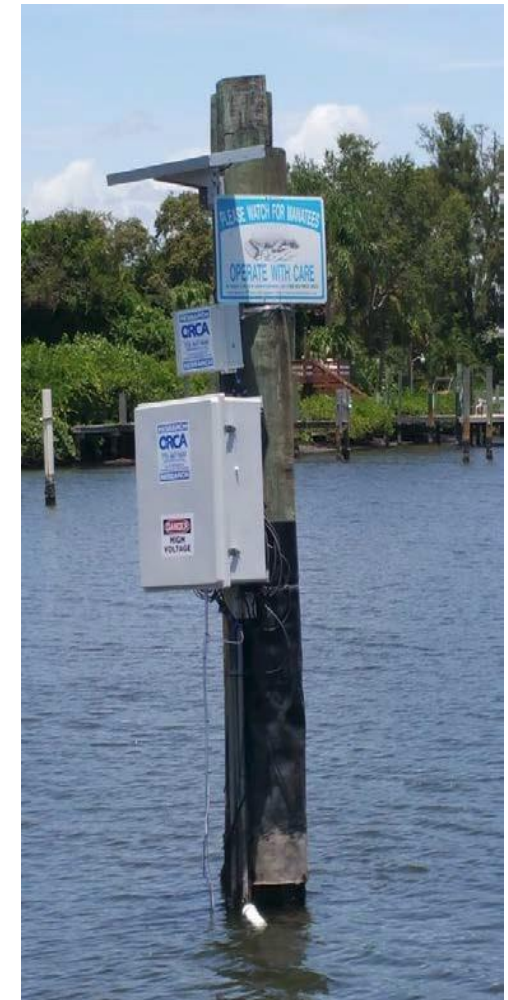
NuLab monitoring nutrients in a waterproof enclosure on a Florida bay
