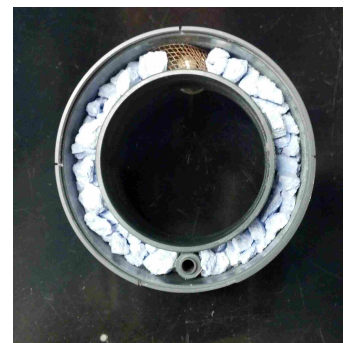
Green Eyes LLC Easton, MD 21601 +1.443.746 info@gescience.com http://www.gescience.com Fig. 4: Biocide Chamber filled with crushed tri-chlor pellets
