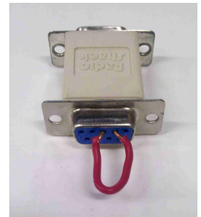
* Com port redirection with a db9 gender changer - pins 2 (receive) and 3 (transmit) jumpered
